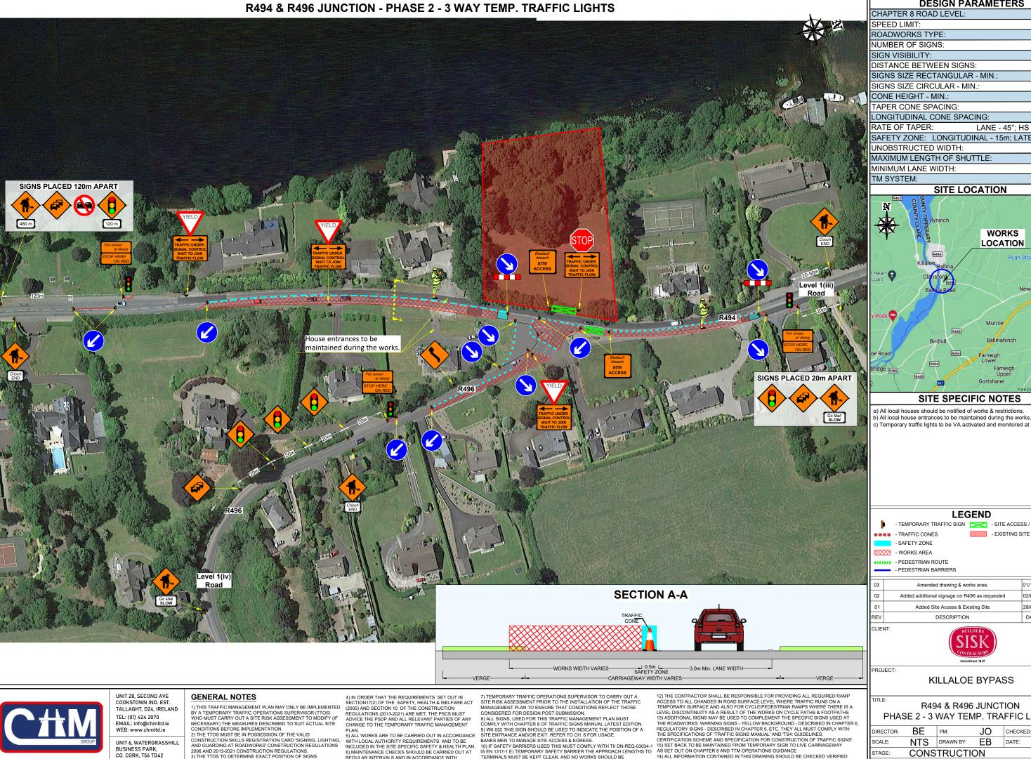
CHAPTER 8 ROAD LEVEL: SPEED LIMIT: 60km/h ROADWORKS TYPE: NUMBER OF SIGNS: SIGN VISIBILITY: 60m DISTANCE BETWEEN SIGNS: 20m SIGNS SIZE RECTANGULAR - MIN.: 600mm SIGNS SIZE CIRCULAR - MIN.: 600mm CONE HEIGHT - MIN. 750mm TAPER CONE SPACING: 3m ONGITUDINAL CONE SPACING: RATE OF TAPER: LANE - 45°; HS - 1 IN 10m SAFETY ZONE: LONGITUDINAL - 15m; LATERAL 0.5m JNOBSTRUCTED WIDTH: MAXIMUM LENGTH OF SHUTTLE: 500m MINIMUM LANE WIDTH: TEMP. T/L TM SYSTEM: SITE LOCATION
