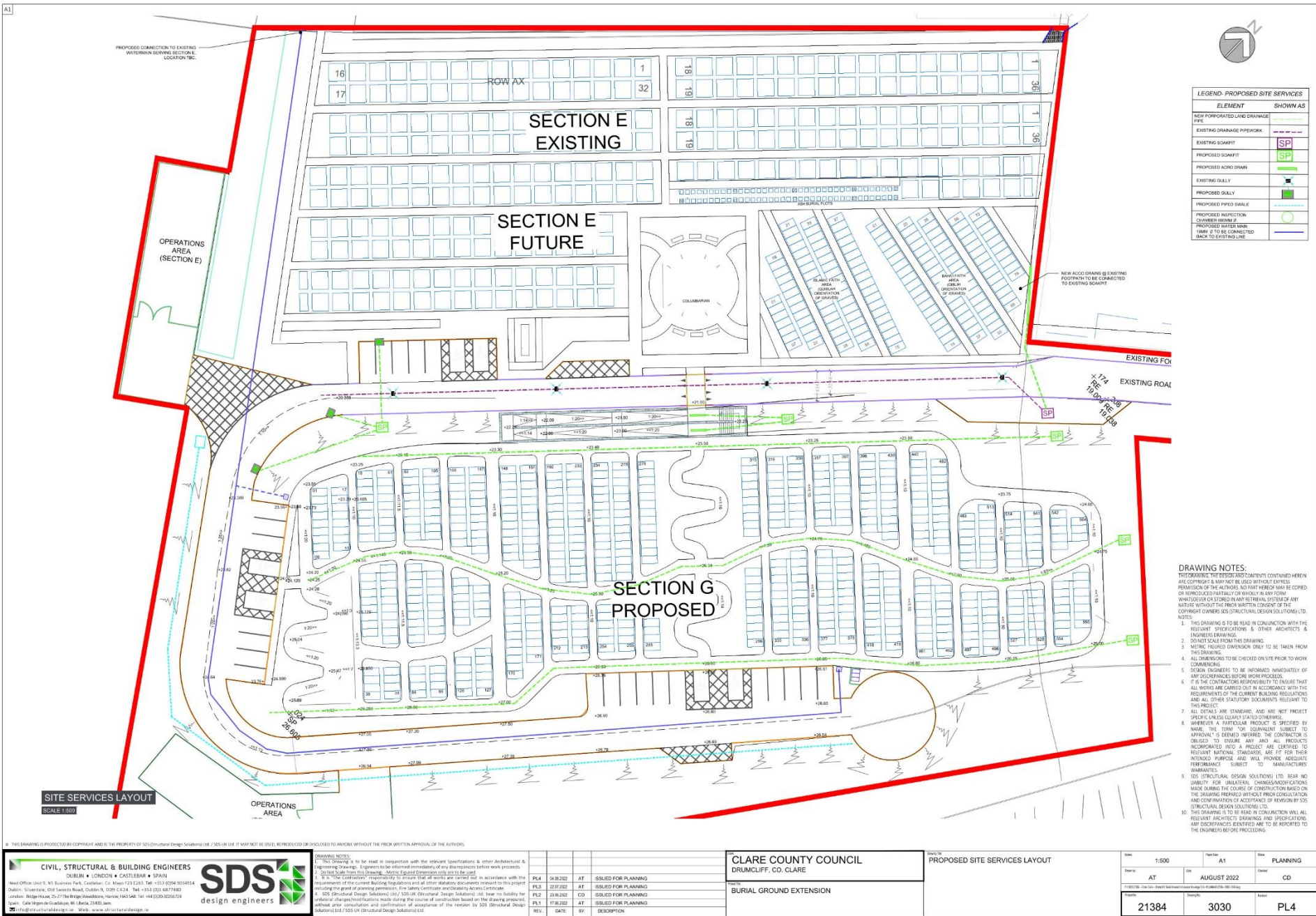
Figure 4. Proposed site services layout
