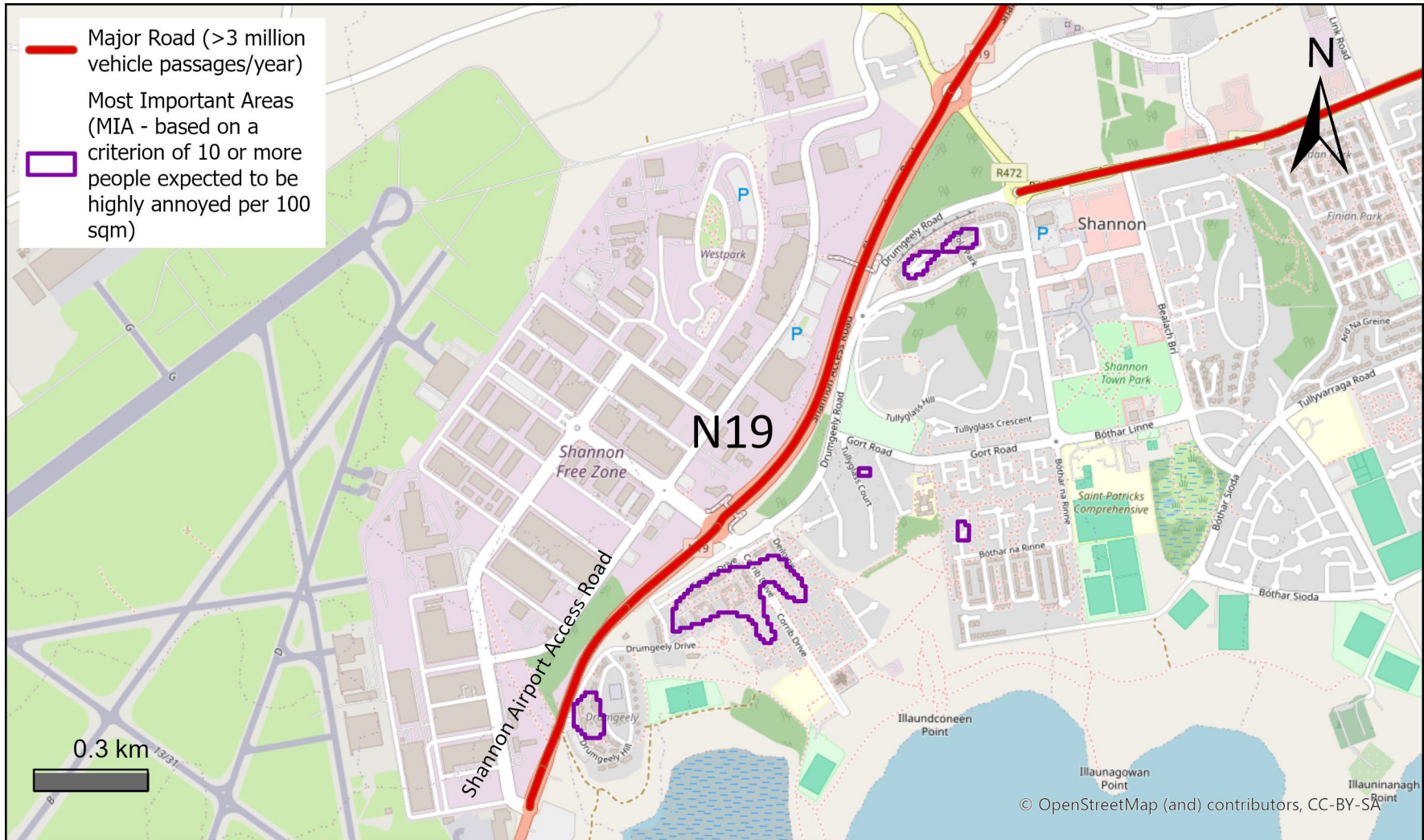
Figure 5.2 : The Shannon PIA with MIAs identified along major road qualifying for strategic noise mapping (N19)
