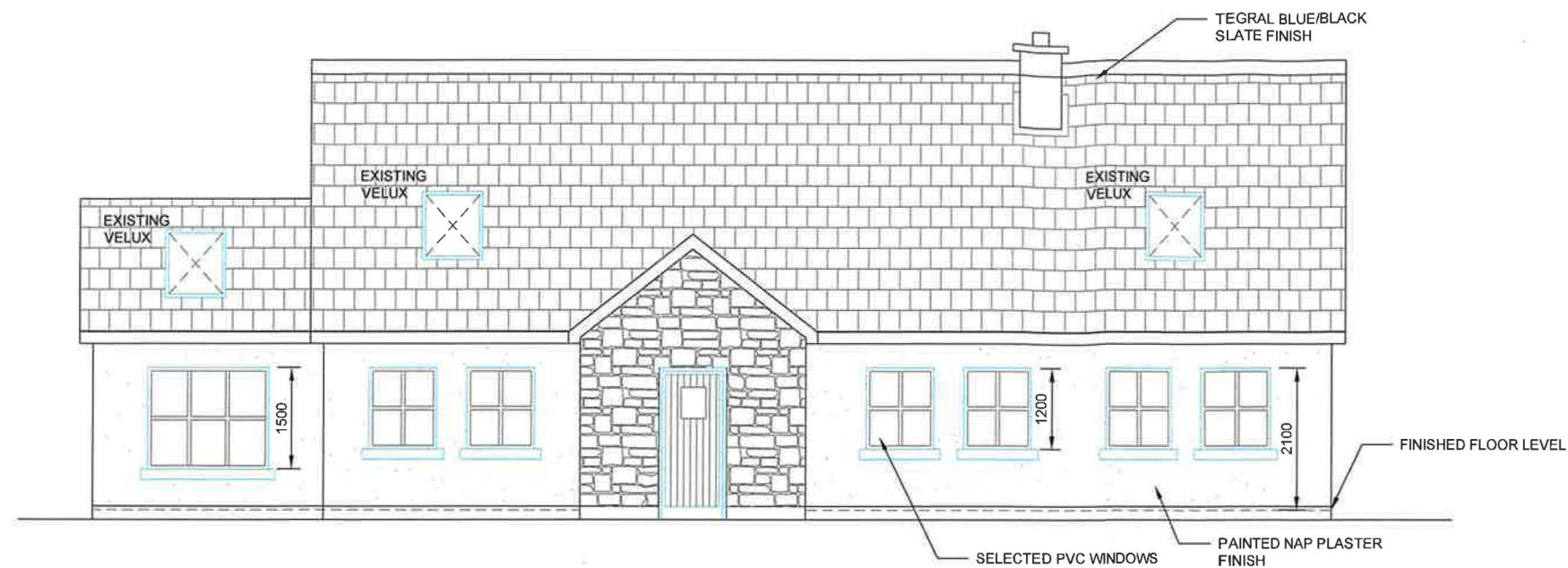
EXISTING FRONT ELEVATION - PLANNING REF 10807
