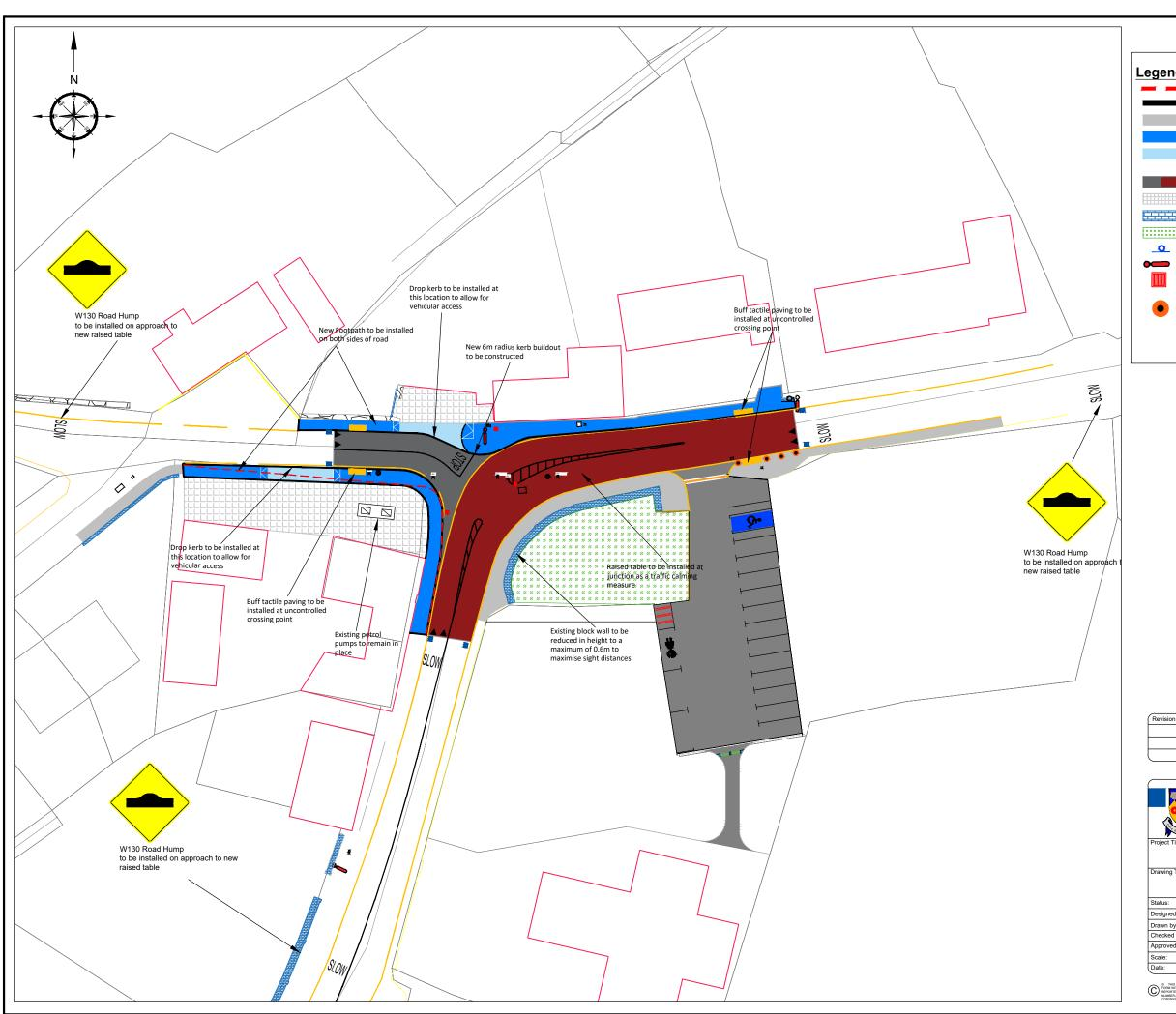
Legend: **Existing Layout** Proposed new kerbing **Existing Footpath** Proposed Footpath Proposed drop kerb at entrance Raised Table Private Property **Boundary Wall** Green Area ...... **Existing Signage** Lamp Post **Existing Road Gully** Flexible Bollards
