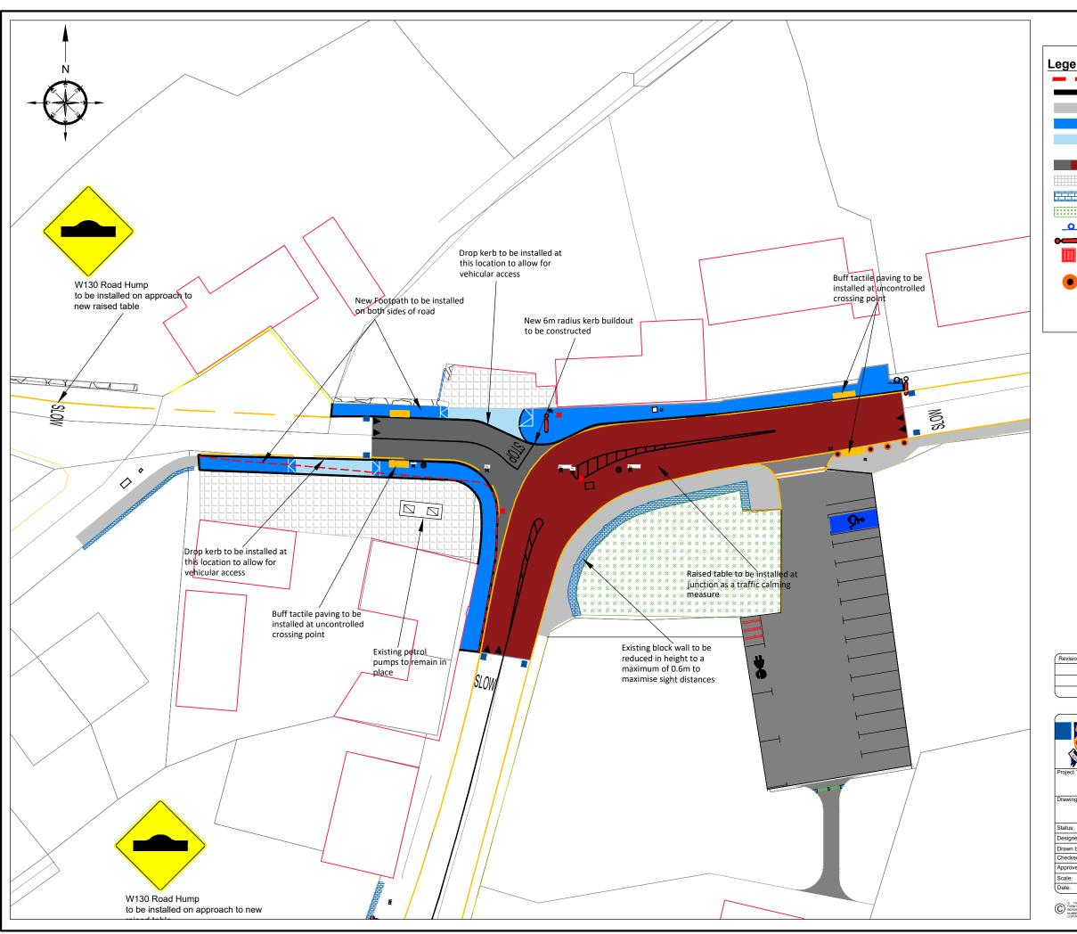
Legend: **Existing Layout** Proposed new kerbing **Existing Footpath** Proposed Footpath Proposed drop kerb at entrance Raised Table Private Property **Boundary Wall** Green Area . . . . . . . . . **Existing Signage** 0 **~** Lamp Post **Existing Road Gully**
